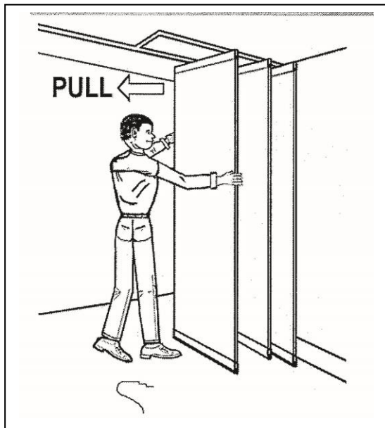
Beginning to extend the panels
