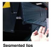
The segmented lips are used to allow the lip to adapt to small and normal trucks.
