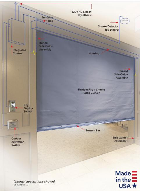
**System Operation.** The system is deployed on an alarm signal from the local smoke detector or from a fire control panel. System power requirement is 120-volt AC. The unit is also equipped with a 24-volt DC battery back-up system that is maintained by the electronic controls. When required, the system can also be connected to building standby power. The controls include a universal power supply that can be adapted to foreign electrical current requirements.
