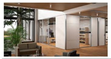
Perfect modular alternative to standard walls Solid partitions utilize 19mm (3/4") faces and high density mineral wool insulation Surface or recessed mounted
